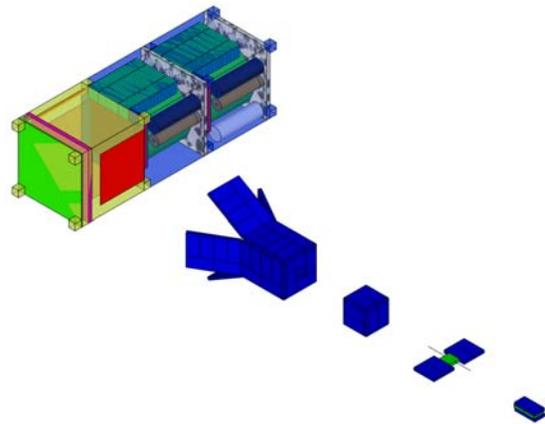
Fig. 4: Example spacecraft configurations that can be printed by a 1U POP and 2U ICES cartridge.
